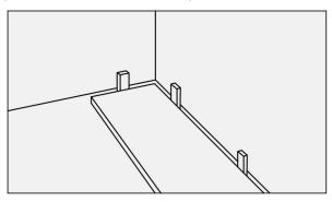
4. Install the second row. Use the offcut from the first row to start the second row. It must be >300mm, and not closer than 300mm from the end join in the previous row.
