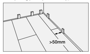
10. Remove spacers/wedges from around the room and install skirting boards and/or scotia and/or finishing trims. Never fix any trims directly to the floor and ensure fixing does not compromise expansion gaps. Silicone or caulking compound is not recommended.
